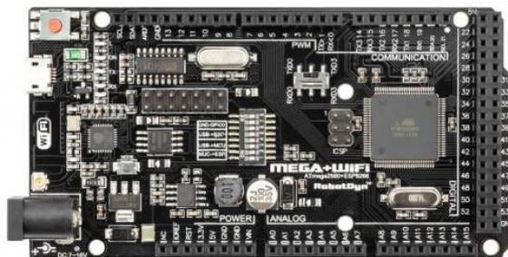
Gambar 2. 1. Arduino Mega 2560
