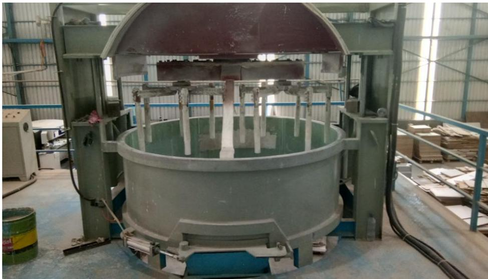
Gambar 3. 7 Mesin *Mixing*
