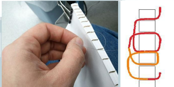
Gambar 2.2. Perfect Binding Step 1 : Kertas dijahit www.instructables.com , n.d.
