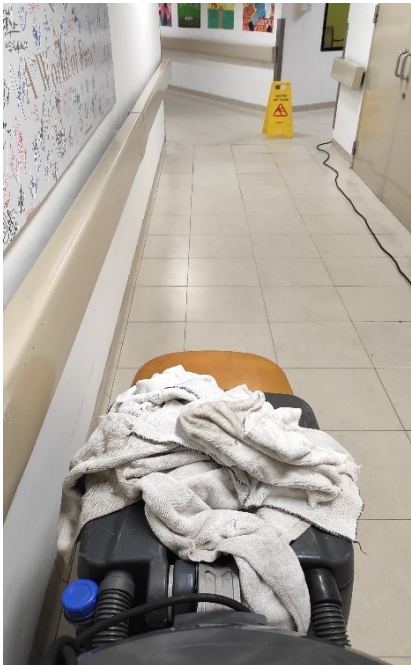
Figure 2.23 Using Swingo floor scrubbing machine
