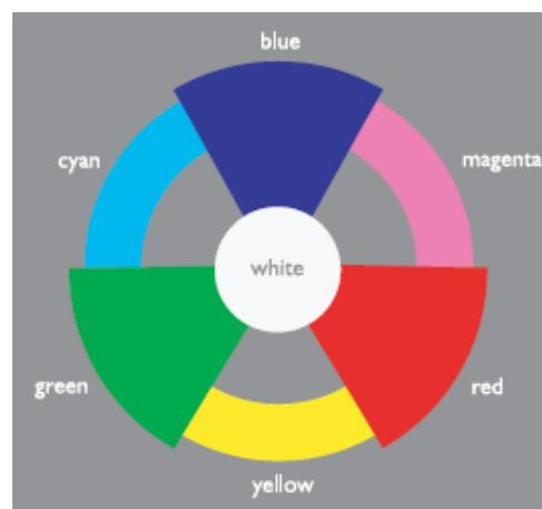
Gambar 2.19. Diagram Warna *Additive* RGB
