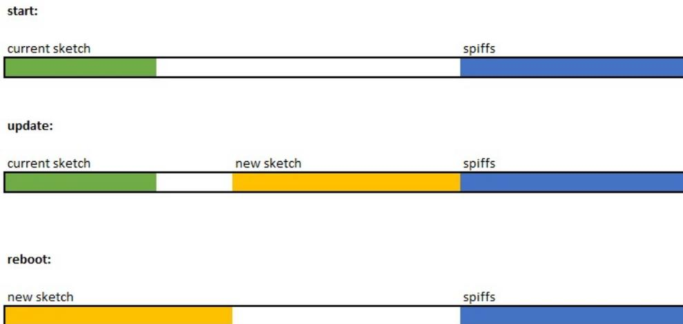
Gambar 3.2 *Flash memory layout* selama proses *atomic firmware update*
