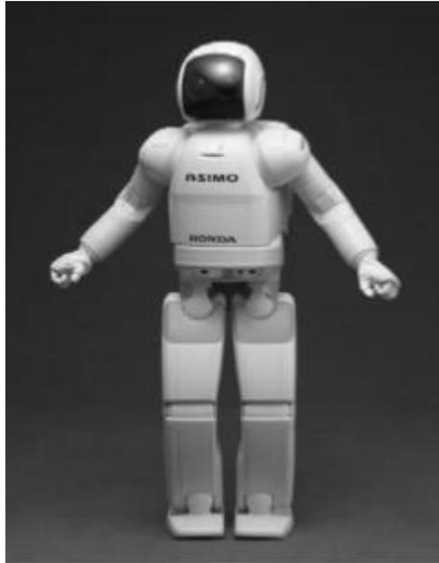
Gambar 2.23. Robot bipedal
