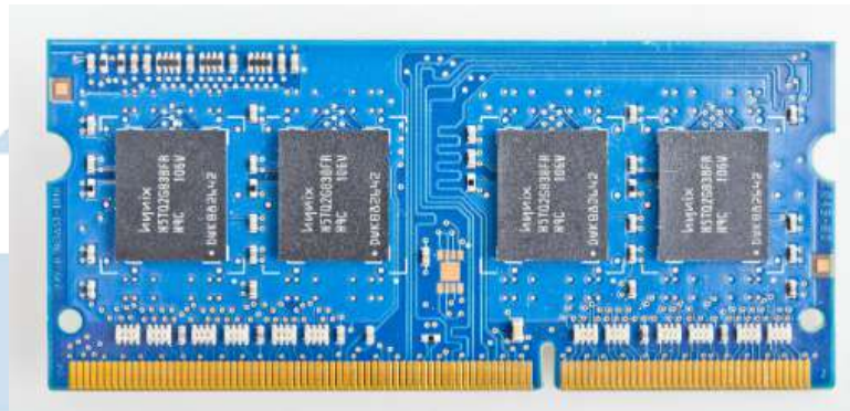
Figure 2.56. Examples of Frontlighting on A Stick of RAM (Source: Thomas, J. D., 2013)
