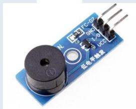
Gambar 3. 16 *Active Piezo Buzzer module*.
