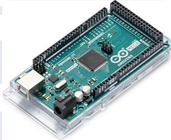
Gambar 3. 12 *Board* Arduino MEGA 2560 R3.
