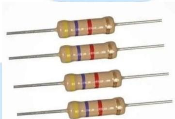
Gambar 3.16 Resistor 4,7K Ohm
