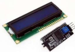
Gambar 3.10 LCD 16x2 I2C
