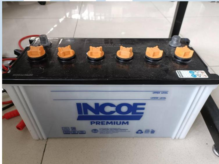
Gambar 2.4 *Flooded Lead Acid*
