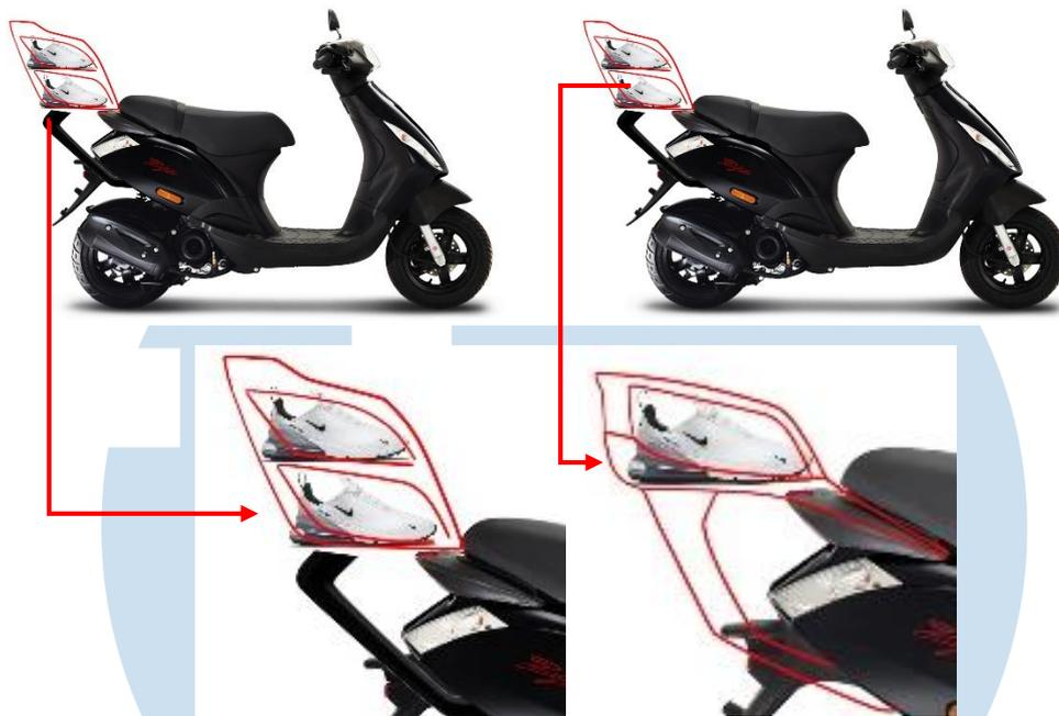
Gambar 3.4 Opsi Sketsa *Custom Rear Shoe Carrier* Motor Piaggio Zip
