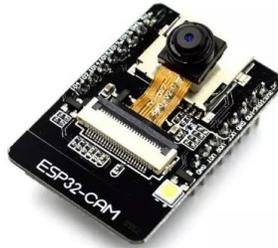
Gambar 2.18: ESP32-Cam with Secure Digital (SD) Cardboard
