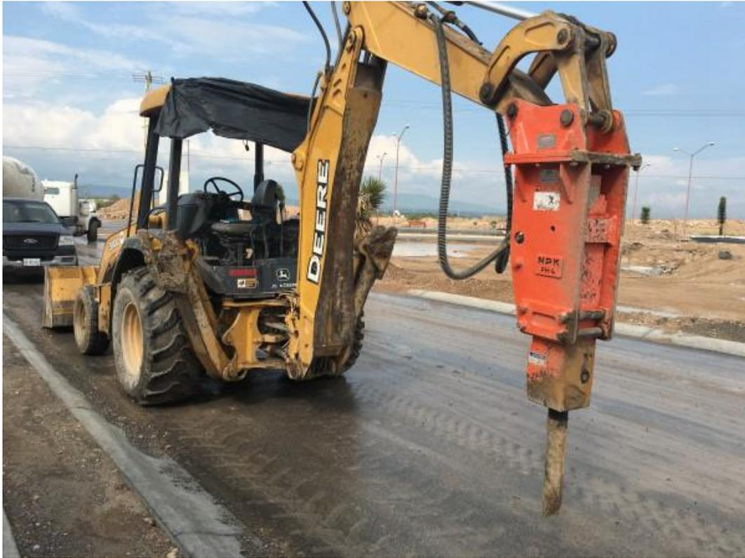
**Gambar 2.3. Hydraulic Hammer**
