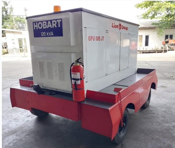
Gambar 3.26. GPU AC/DC 120 kVA
