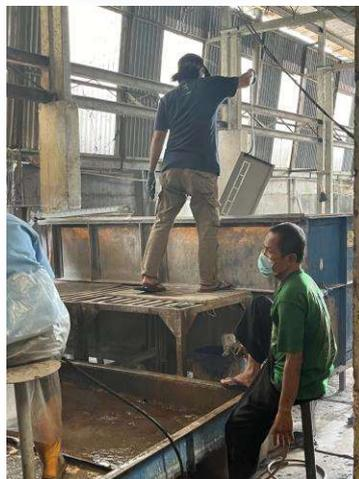
Gambar 3.18 Proses *Phosphate* Rangka Panel
