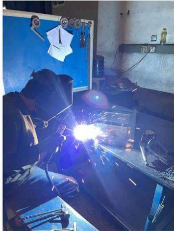
Gambar 3.15 Proses Las Rangka Panel
