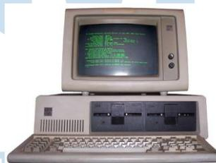
An early IBM PC with two floppy disk drives. PCs could be purchased with a single floppy drive, or with a hard drive in place of a floppy drive.
