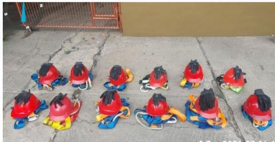
*Gambar 3. 17 Working Belt, Helm, Sepatu*
