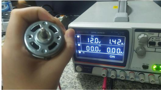
Gambar 3.19 Pengujian Motor DC *High Speed*
