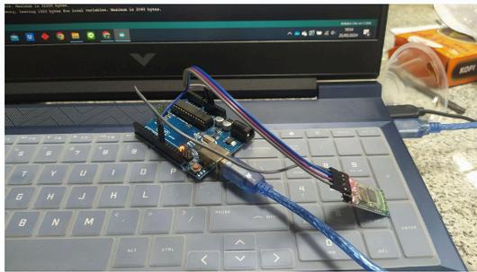
Gambar 3.14 Pengujian Bluetooth *Transceiver* HC-05
