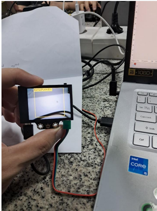
Gambar 3.3 Pengujian object identification Huskylens SEN0305
