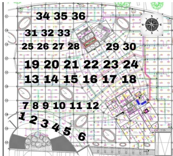
Figure 3.7 Tower D Basement Measurement Points
