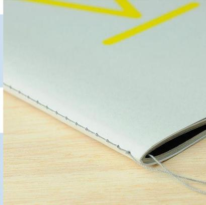
Gambar 2.45 *Thread Sewing Binding*
