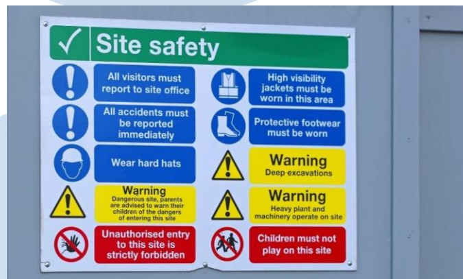
Gambar 2. 3 Contoh Penggunaan Signage Sumber: https://www.tfs.com.au/wp-content/uploads/2020/04/tfs-importance-workplace-safety-signage-construction-sites.jpg
