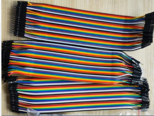
Gambar 3.9 - Kabel jumper
