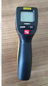
Gambar 3.13 - Termometer *infrared*
