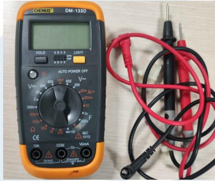
Gambar 3.14 - Multimeter
