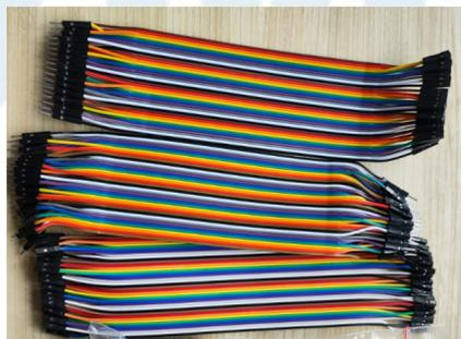
Gambar 3.8 - Kabel *jumper*
