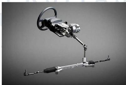
Gambar 2.28 *Electric Power Steering*
