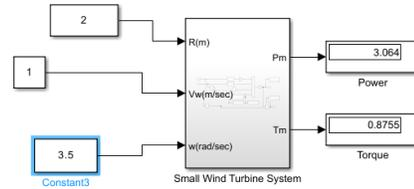
Fig. 3. Small Wind Turbine System Sample Model
