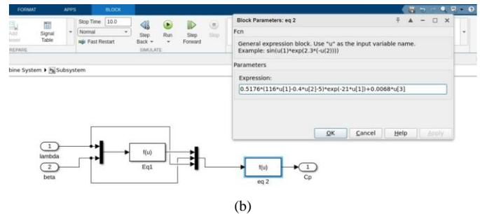
Fig. 2. System for exponential and sinusoidal model a) Breakdown for Exponential and Sinusoidal Model for Small Wind Turbine and b) The Subsystem Adjustment According to the Input for  $C_p$
