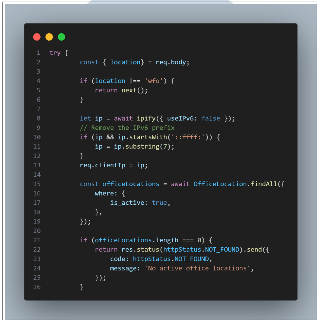
Gambar 3.54. IP checking mechanism
