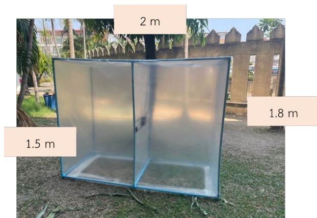
Fig. 1: A laboratory setup for capturing PM 2.5 dust particles.
