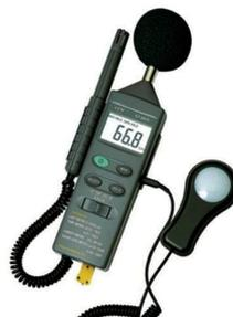
Gambar 3.5 Alat Ukur Environment Meter
