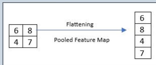
Gambar 2.6. Proses flattening sebelum masuk ke *fully-connected layer*
