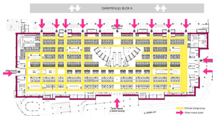
Fig. 28 Entry Access and Circulation Flow for Block B. Source: Reproduction of Tanah Abang Market Block B Plan
