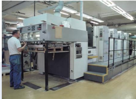
Gambar 2.13 Sheet-Fed Offset Printing Press Sumber: Johansson et al. (2011)
