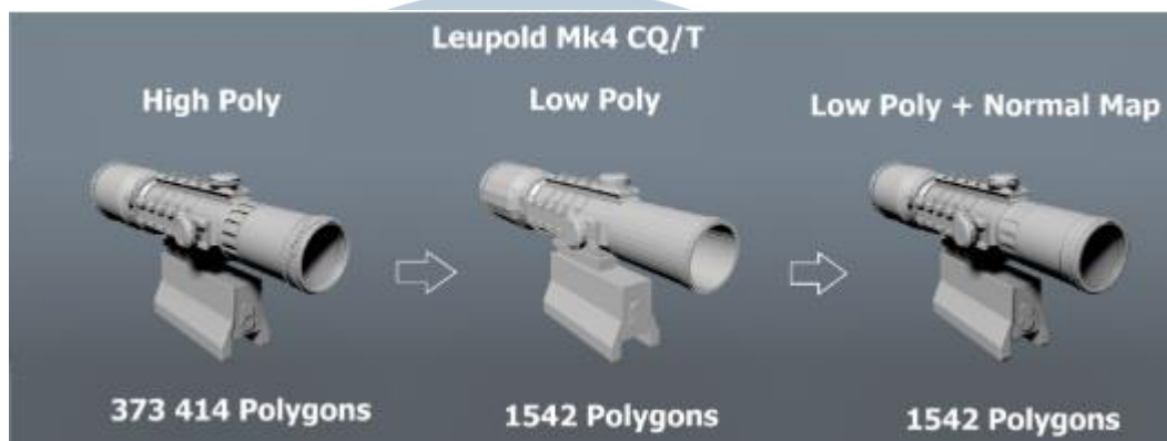
Gambar 2.6. Contoh Model 3D High Polygon dan Low Polygon untuk Game ( http://1.bp.blogspot.com/-peONqYXn_aE/Vk7cly2UiNI/AAAAAAAAABL8/1X_-H0BjjU/s1600/266963_367010970057889_1979841288_o.png )
