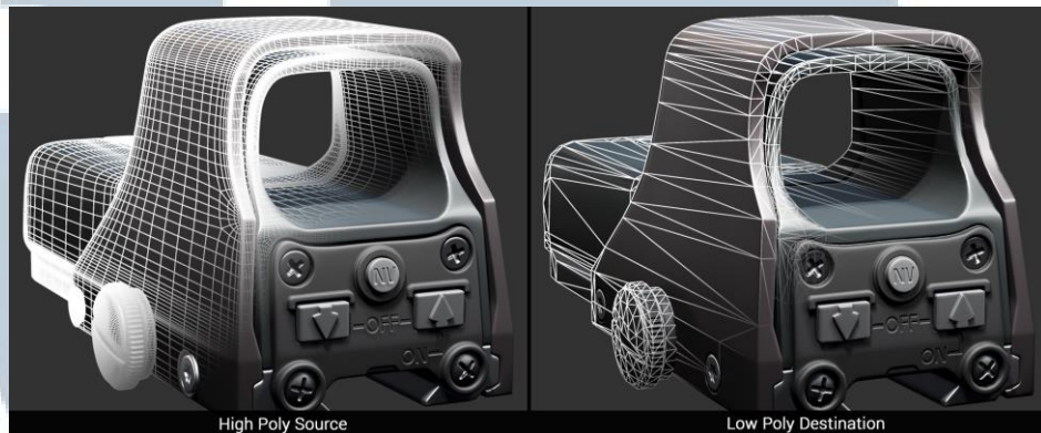
Gambar 2.12. Perbandingan High Poly Modelling dan Low Poly Modelling ( https://www.marmoset.co/wp-content/uploads/2017/04/eotechhighlowb.jpg )
